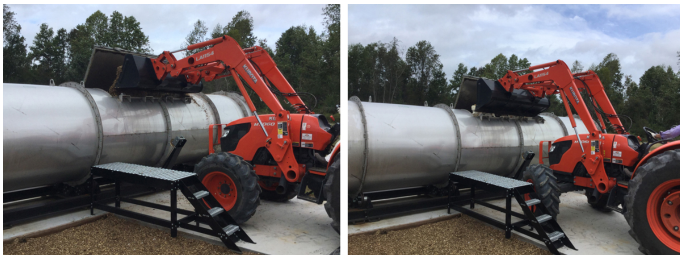
Figure 5. A front-end loader loads the carbon material (A) and the carcasses (B) into a composter.
