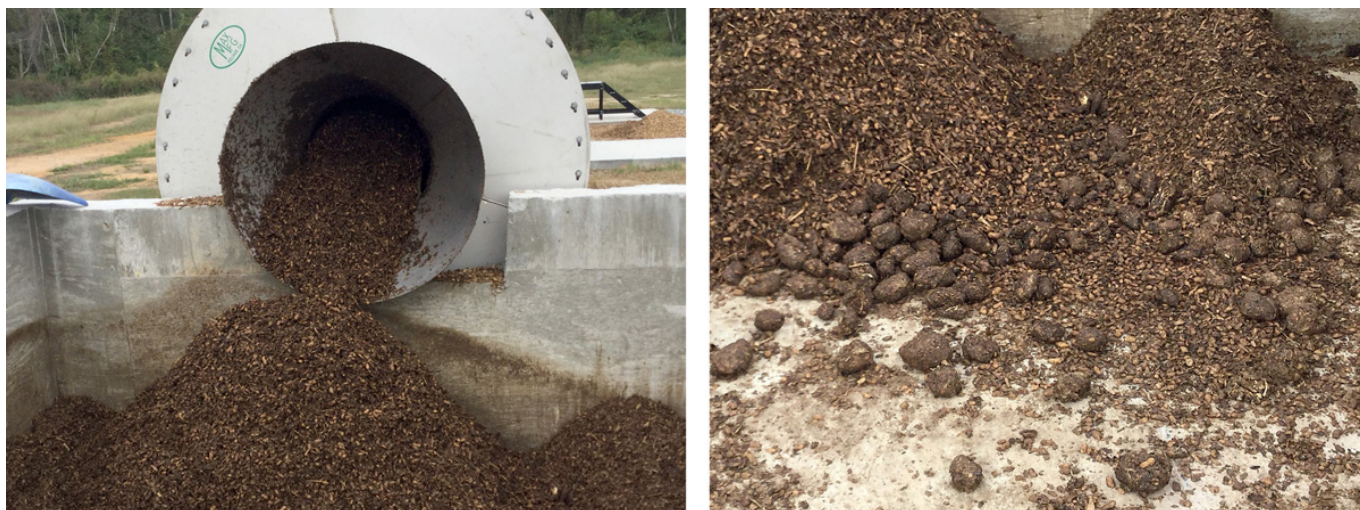
Figure 8. Composter exit materials after 10 days (A). Balls of “cooked” breast meat (B).
