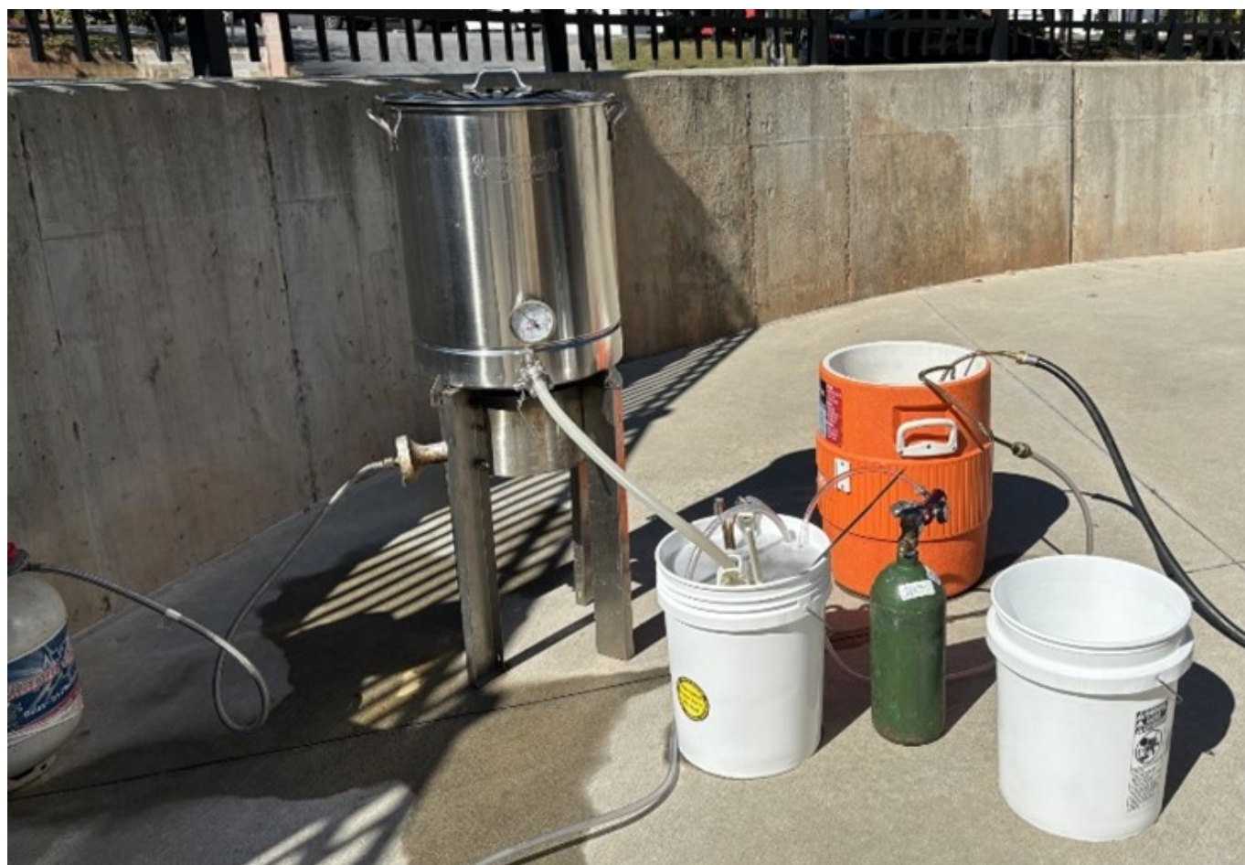
Figure 6. Homebrew Equipment to Brew Wort for Scaling Up Wild Yeast Fermentations.
