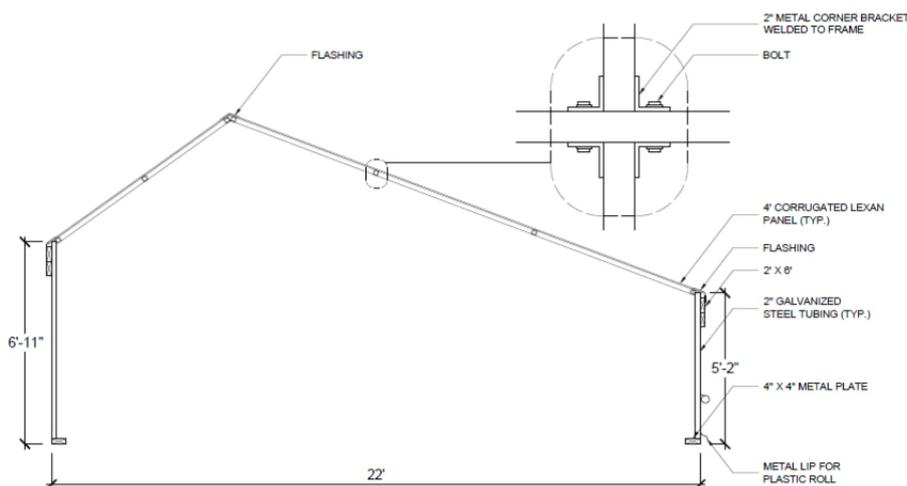
Figure 6. Schematic of the Bows with a Side View of the Structure. Image created by Helen Turner, University of Kentucky, College of Design.
