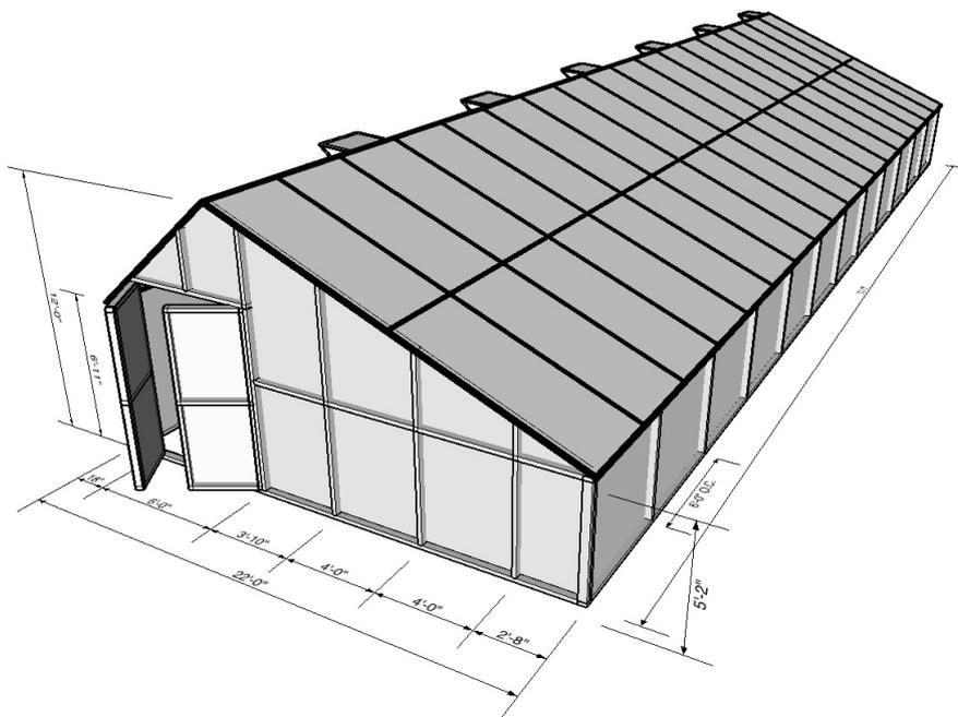
Figure 3. Rendering of the Passive Solar Greenhouse (PSG) Structure Built by the Authors. The primary roof and front wall faced south to absorb the most radiation during the day. Image created by Helen Turner, University of Kentucky College of Design.
