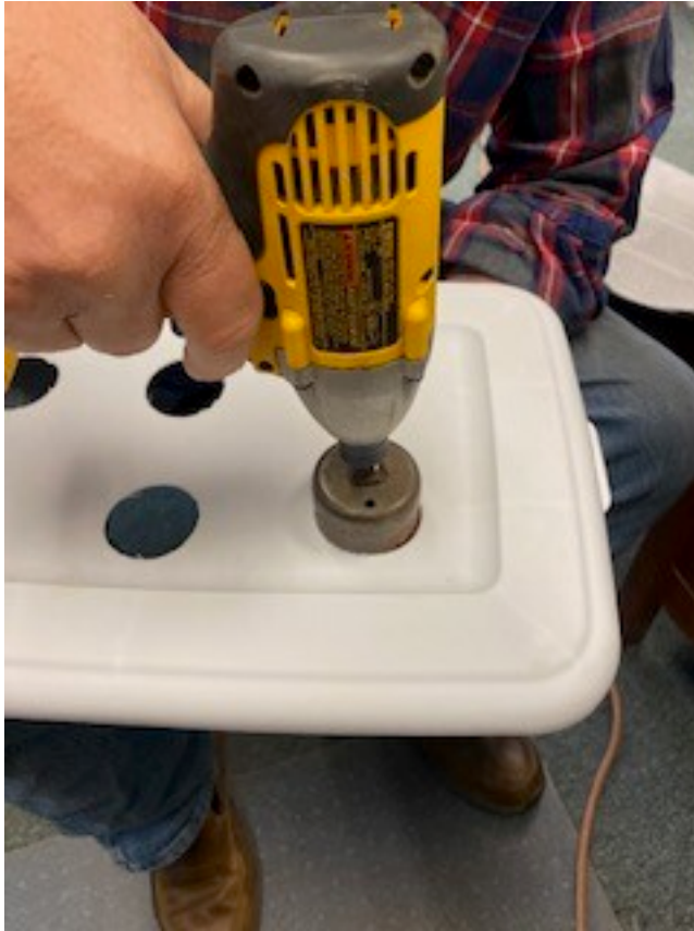
Drilling holes for hydroponic net pots.
