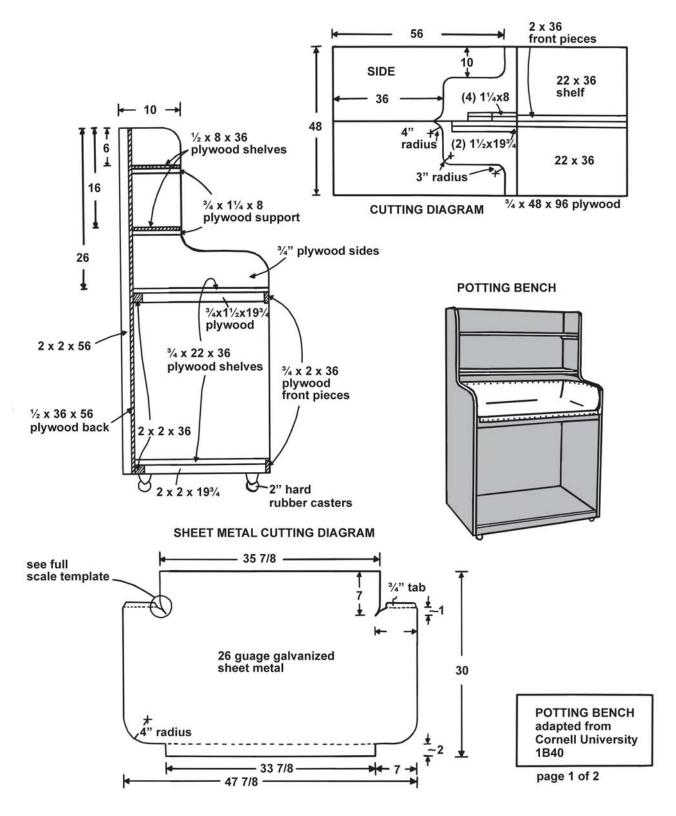
Bend on dotted lines with sheet metal brake or clamp in 2 x 4s & bend over with block of wood & hammer.
