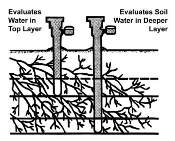
Figure 2. Typical Tensiometer Location
