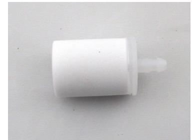
Figure 8. Most two-cycle motors have a small barrel fuel filter inside the gas tank. These should be changed at least once a season.
