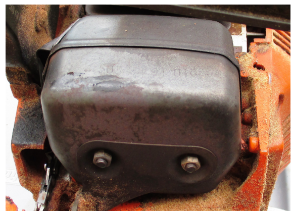
Figure 3. Some mufflers contain spark screens, which must be kept clean to allow for the exhaust flow.
