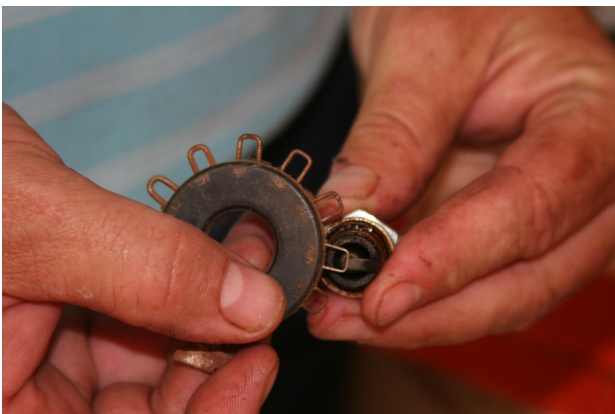
Figure 5. New spark plugs must be set to the proper gap using a spark plug gauge tool.
