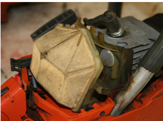
Figure 2. Air breathers should be cleaned on a regular basis by using either compressed air or soap and water on foam elements.
