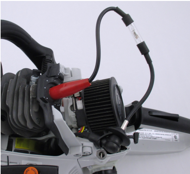
Figure 4. Ignition tester used to check spark plugs.
