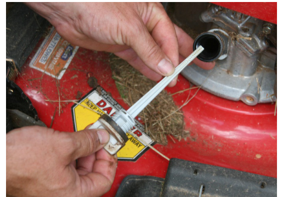
Figure 1. Engine oil should be checked every time before you use your motorized equipment.
